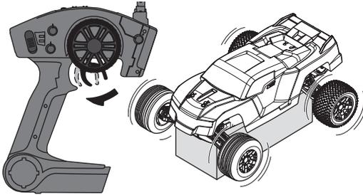
4. Start driving slowly, and, if the vehicle does not go straight, adjust the steering trim dial on the transmitter.
