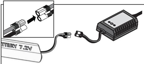
The vehicle battery charger produces 2000 milliAmps (2 Amps) per hour. Divide the mAh capacity on the label of a battery by 2000 to know how long battery charging will require. For example, a fully discharged 1800mAh battery requires 0.9 hours (54 minutes) to charge.
