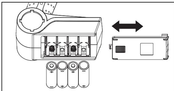
1. Slide the panel open on the bottom of the transmitter.
